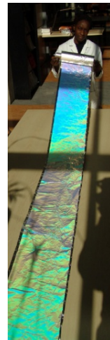
Monolayer of 1 micron SiO 2 beads for pearlescent effects
